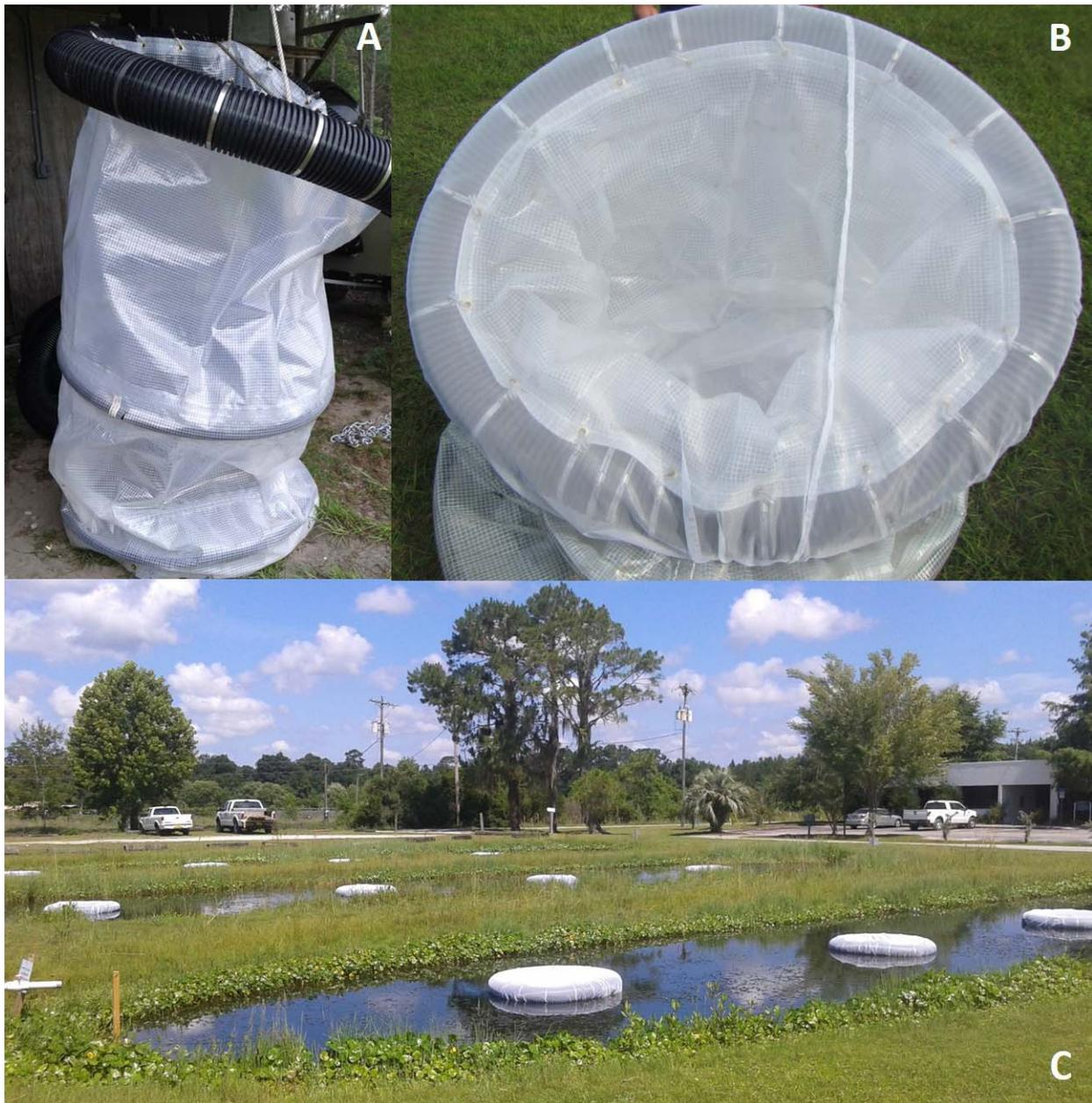
Figure 1. Limnocorrals (1 m diam. by 2 m potential depth) constructed for the experiments (A). A polyethylene tube was suspended from a buoyant PVC pipe ring. A chain at the bottom provided anchorage into the sediment and two PVC pipe hoops provided shape. A net was placed over the top to prevent access of herbivores (B). Four limnocorrals were placed in each of three hydrilla-infested ponds (C). One treatment was randomly placed per limnocorral in each pond.
