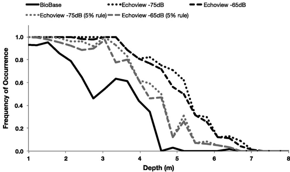
Figure 6. Frequency of submerged macrophyte occurrence for the zigzag tracks on Elk Lake using two hydroacoustic systems. Two target strength thresholds (–65 and –75 dB) were used for the Echoview system. The 5% rule within Echoview represents the application of a 5% threshold rule for vegetation presence similar to the algorithm applied to BioBase data.
