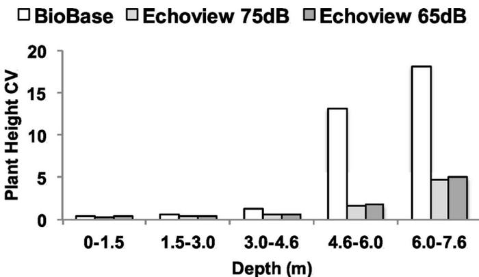
Figure 4. Plant height coefficient of variation (CV) by depth strata for the zigzag track on Elk Lake using two hydroacoustic systems. Two target-strength thresholds ( $-65$  and  $-75$  dB) were used for the Echoview system.
