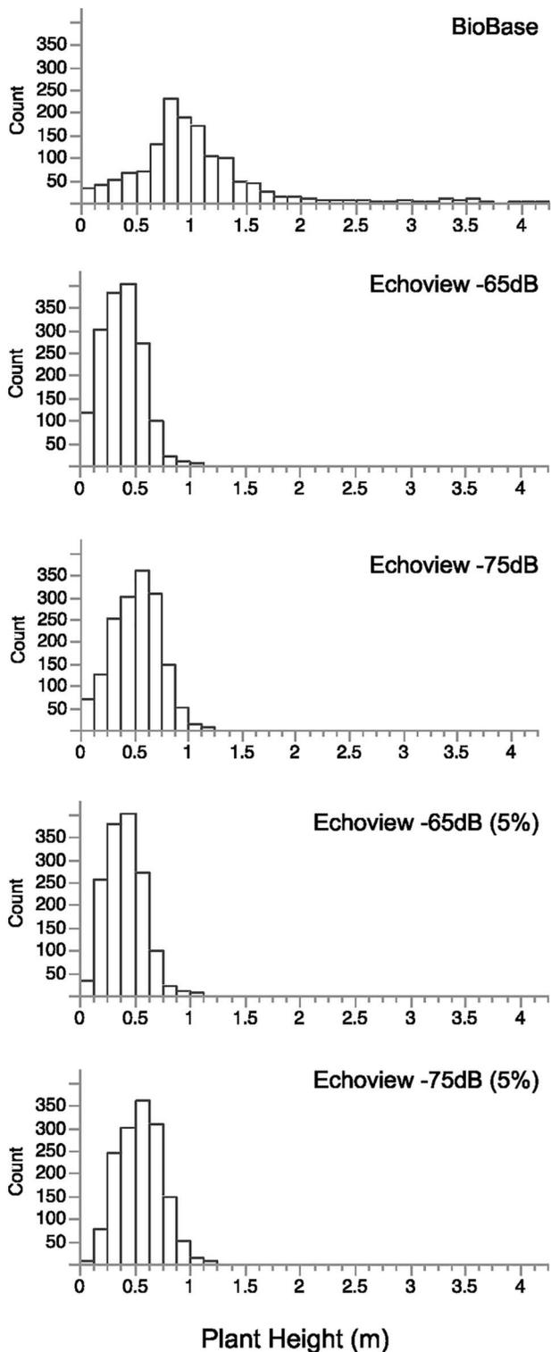
Figure 5. Plant height frequency distributions for the zigzag track on Elk Lake using two hydroacoustic systems. Two target-strength thresholds (–65 and –75 dB) were used for the Echoview system. The 5% rule within Echoview represents the application of the BioBase 5% threshold rule for the vegetation height to water depth ratio within the Echoview system.
