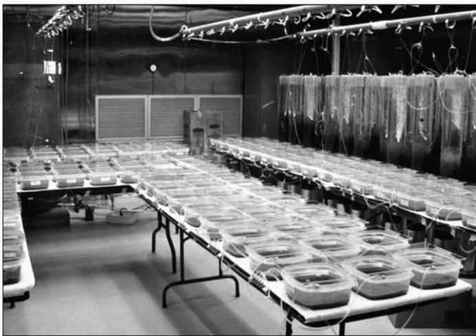
Figure 1. Set-up showing direct application of seedling emergence method in an environmental growth chamber at the US Army Engineer Research and Development Center (ERDC), Vicksburg, Mississippi.
