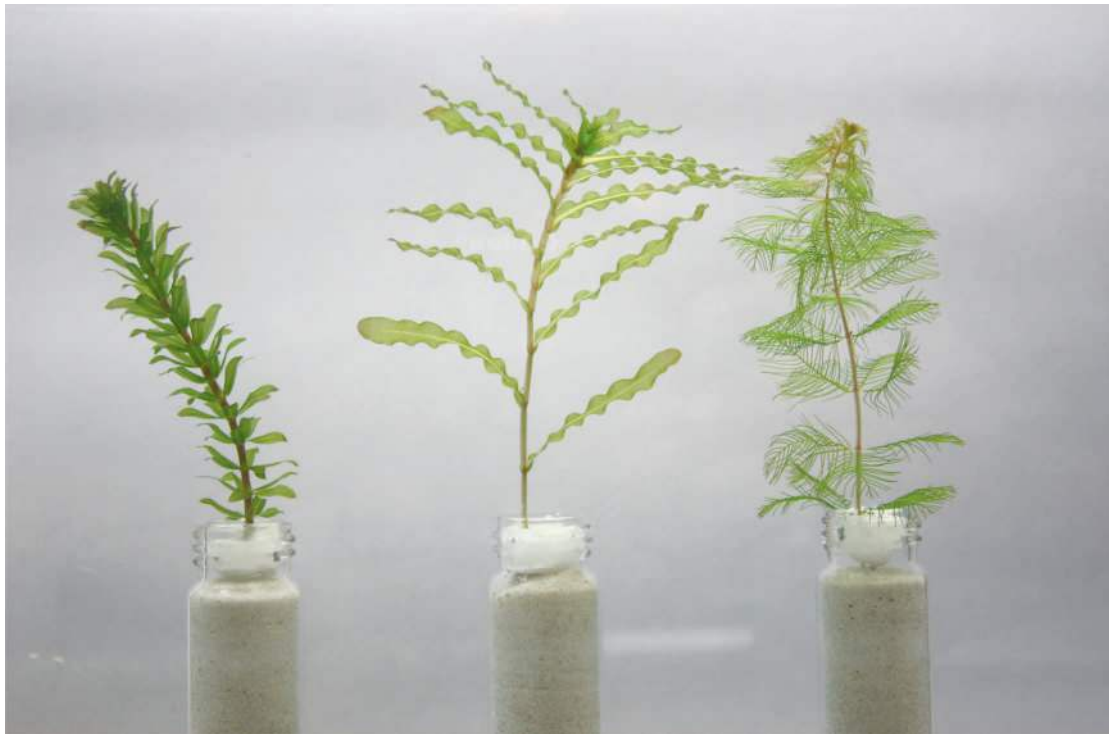
Figure 3. Hydrilla, curly leaf pondweed, and hybrid watermilfoil apical shoot cuttings were grown for several weeks to develop adventitious roots and transferred to vials filled with fine, washed silica sand. Plants were allowed to acclimate for several days before treatment. The white material at the top of the glass vial is eicosane wax. (Frank and Hodgson 1964) (courtesy M. Ortiz, Colorado State University).
